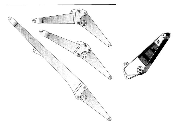
**2 piece main boom** with pin-mounted joint between boom foot and boom nose.
