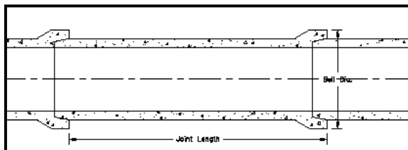
Typical Concrete Pipe Configuration
