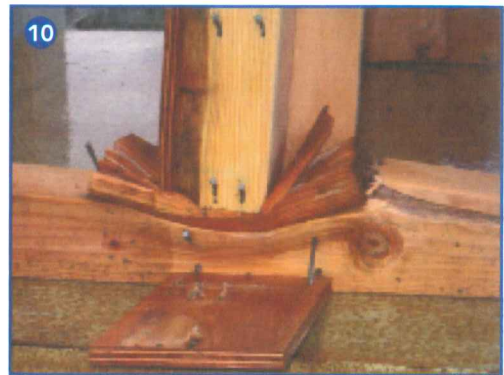
(9) The final version of the 2-foot × 4-foot PLP at failure. The posts fractured at knots and the headers and soles gave ample warning of failure as they were crushed and split. (10) PLP-85 after failure, showing extent of crushing of sole, and cupping of wedges. The failure load was 140k (4.4 times design load), which is attributed to the uniform straightness and absence of knots in all four posts.
