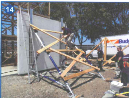
(11) Typical test setup for testing a pair of solid sole rakers. (12) Raker pair after sole cleat fly-off; nails were reduced to only six. (13) Pneumatic raker system with lateral bracing. (14) Test of redesigned pneumatic raker.
