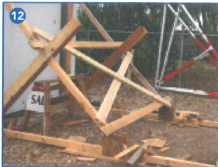
(11) Typical test setup for testing a pair of solid sole rakers. (12) Raker pair after sole cleat fly-off; nails were reduced to only six. (13) Pneumatic raker system with lateral bracing. (14) Test of redesigned pneumatic raker.
