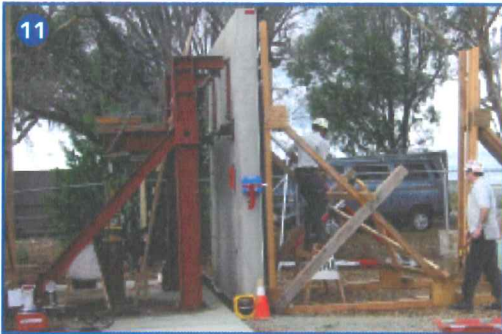
(11) Typical test setup for testing a pair of solid sole rakers. (12) Raker pair after sole cleat fly-off; nails were reduced to only six. (13) Pneumatic raker system with lateral bracing. (14) Test of redesigned pneumatic raker.
