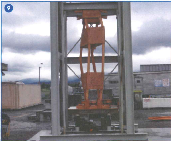
(9) The final version of the 2-foot × 4-foot PLP at failure. The posts fractured at knots and the headers and soles gave ample warning of failure as they were crushed and split. (10) PLP-85 after failure, showing extent of crushing of sole, and cupping of wedges. The failure load was 140k (4.4 times design load), which is attributed to the uniform straightness and absence of knots in all four posts.
