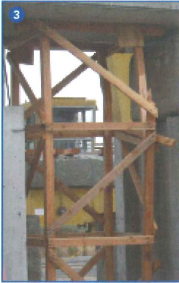
(3) The typical conditions at failure. Test specimen LP-31's right-front post split at a knot near the intersection of the upper mid-brace and two diagonals. (4) At the upper right, the right-front post has crushed the header to about half its thickness, which displaced the then-standard 12 x 12-inch full gusset. The standard now recommends using 6 x 12-inch half-gussets, which are quicker to install and allow a better view of the crushing of the header. (5) The right-front post at failure load (3.2 times the design load) crushed the wedges and caused them to cup. Crushing and cupping are quite obvious at about two times the design load and indicate that shore is overloaded and personnel must take action.
