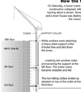
While workers were attaching a heavy steel support collar it broke free and slid down the tower ...
